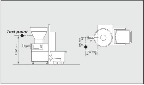
Noise measurement for straight stuffing without twisting with 100% filling speed without product with sound level meter (DIN 45 634) < 80 dB(A)
