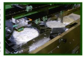
which is elevated up and over the first product onto a "holding platform." When both products are aligned with each other, they are swept forward by the overhead paddle in a one-on-one format. The stacked product is then automatically timed into the awaiting flights of the product infeed conveyor.
