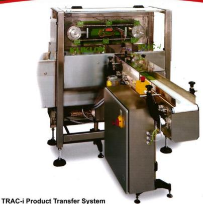
The independently driven "Transfer Right-angle Auto Collator" (TRAC-i) is designed to provide collation and transfer of products into the continuously running infeed conveyor of end-load cartoning machines. The servo design, rugged construction and compact footprint provides layout and application flexibility. Special configurations allow cost effective product stacking and
